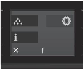
The **JURA Cockpit** allows you to manage your X10. Press the > button for **approx. 2 seconds** to enter the JURA Cockpit.
