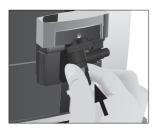
► Fit the assembled individual parts back in the dual spout and press it firmly.
