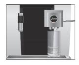
Coffee preparation starts. The preset amount of water for espresso flows into the glass. Preparation stops automatically. Your GIGA is once more ready for use.
